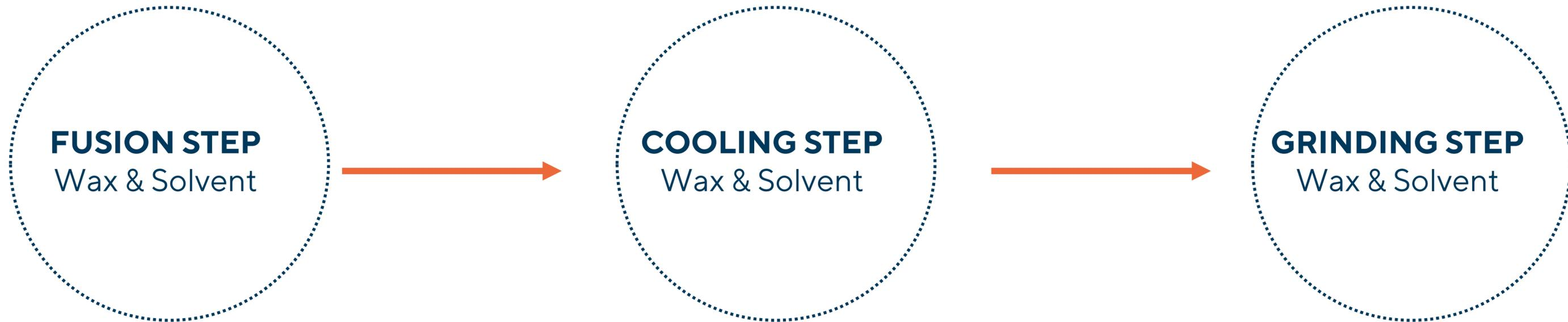
Temperature is increased over wax melting point and once wax is completely melted it is mixed with solvent under stirring.
